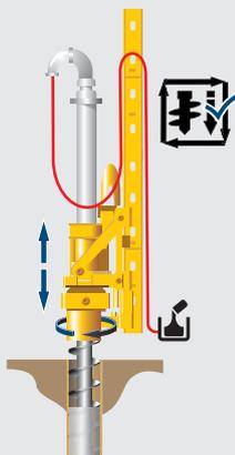
**Automatic drilling and extraction control – single pass**
