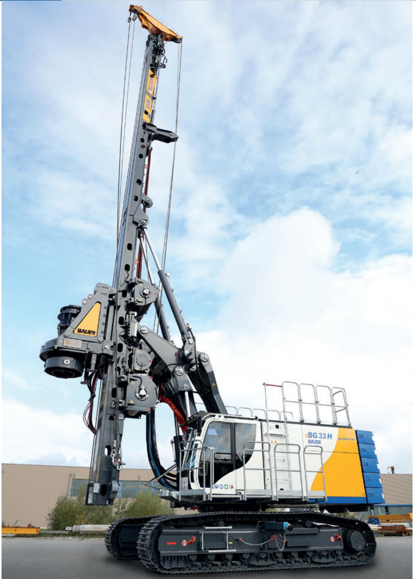
The Bauer drilling rigs are multi-function equipment for a wide range of construction methods in specialist foundation engineering. Of course this is also true for this highly modern fully electric variant.
