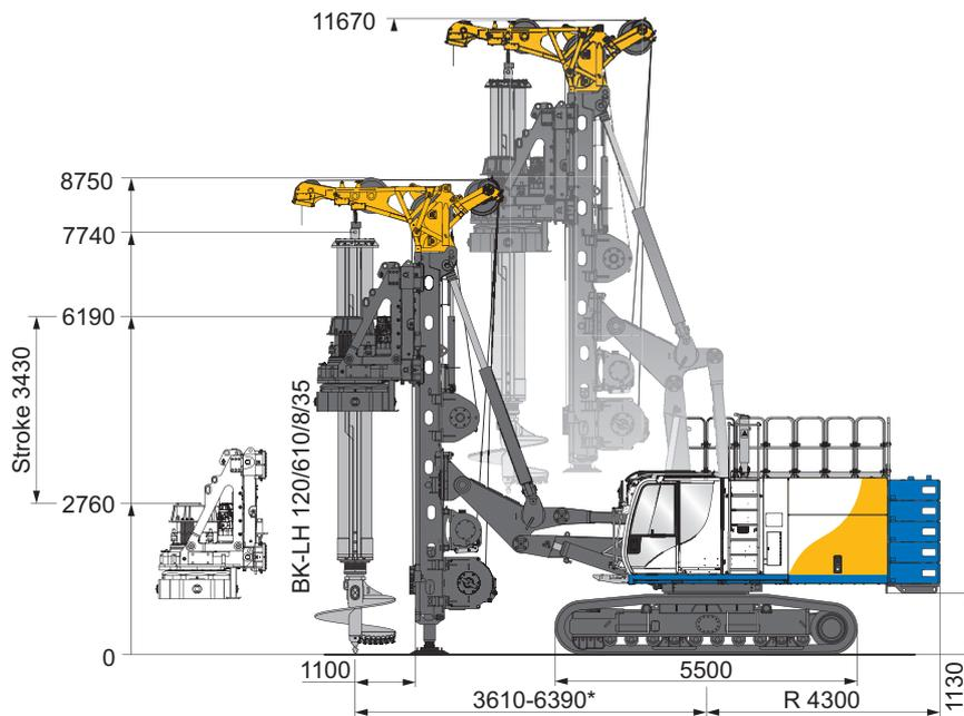
Low Headroom system for large drilling depths
