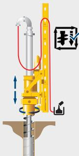
**Automatic drilling and extraction control for Single-Pass processes**
