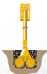
CSM Cutter Soil Mixing
